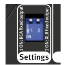
DIP switch 1: OFF = The level of the RCA analog output is adjusted with the volume control.
